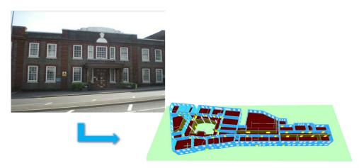
Figure 3: screenshot from iBuildNet providing a 3D view of coverage simulation in a building
